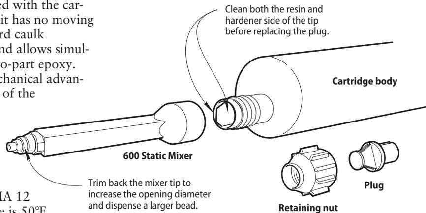
Remove and save the retaining nut and plug to reuse if you are storing the unused adhesive. Be sure the plug is replaced in the original orientation to avoid cross contamination. Mark the plug and cartridge to avoid confusion.
